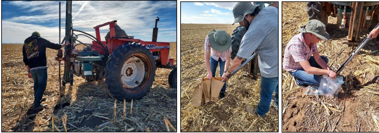
Plates 7,8 & 9. Using a tractor-mounted hydraulic probe to extract soil samples at profile depth for carbon analysis in northern Dallam County, 2022.
