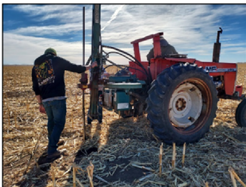
Images 6,7,8. Using a tractor mounted hydraulic probe to extract soil samples at profile depth for carbon analysis in northern Dallam county, 2022.
