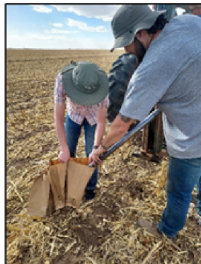
Images 6,7,8. Using a tractor mounted hydraulic probe to extract soil samples at profile depth for carbon analysis in northern Dallam county, 2022.
